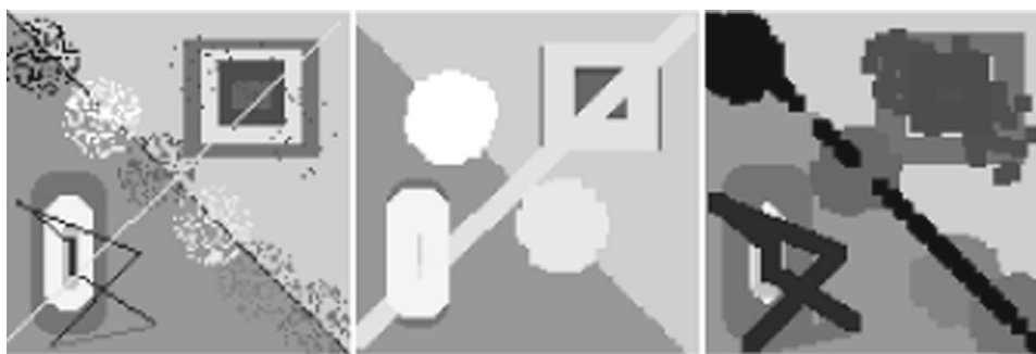
Fig. 6 Standard (MATLAB) greyscale dilation and erosion with a flat 5 \times 5 SE. From left to right: Original image, dilated image and eroded image
