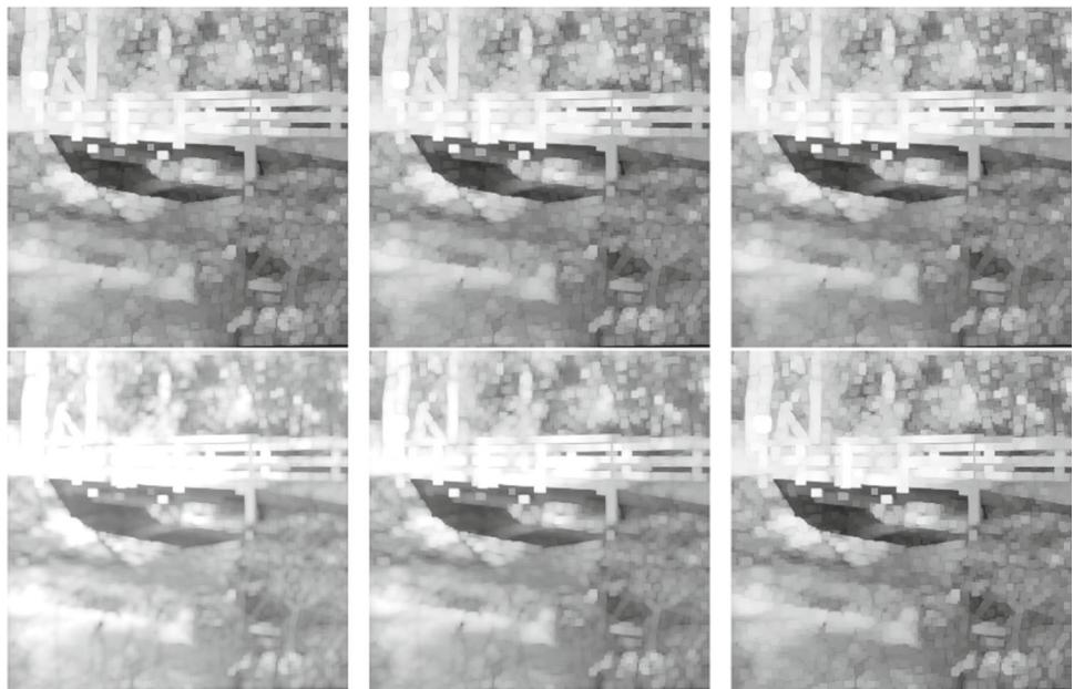
Fig. 4 Comparison of filtering results for dilation of the 256 \times 256 bridge image with a 5 \times 5 mask. Top: From left to right: Exactly dilated image, approximately dilated image with factor n = 3.5 and n = 2.5 . Bottom: From left to right: Approximation with scaling factor 0.05, 0.1 and 1
