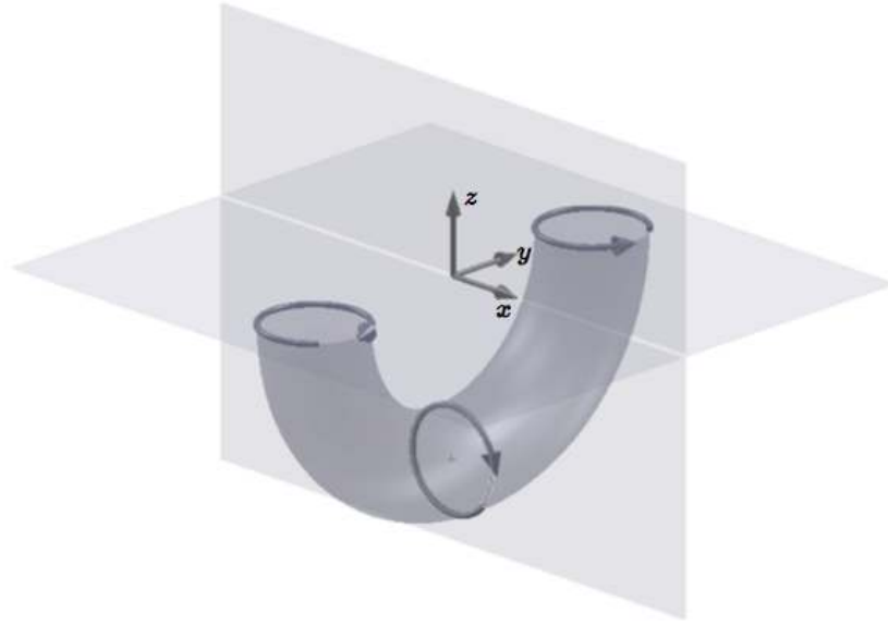
Figure 2.4: Description, proposed by Peregrine (1999), of the topological shape (a half vortex ring) of the flow shortly after a breaking event. The surface of the torus denotes the vortex filament and the arrows indicate the direction of the velocity.
