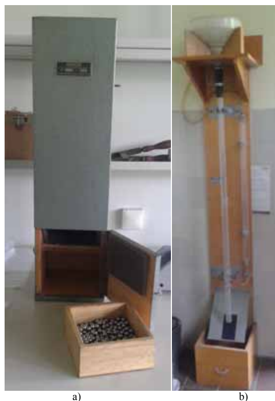
Figure 3. Erichsen 273 D device for test of resistance to steel balls impact (a), and Erichsen 251/I device for abrasion resistance test (b)
