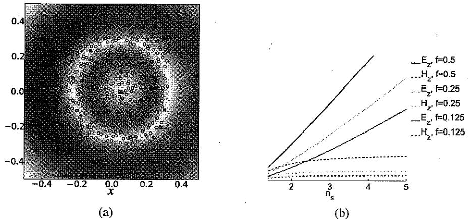
Fig. 6. (a)  $\text{Re}[H_z]$  component of time-reversed field for  $H_z$  polarization, for parameters of Fig. 3(a). (Note change in scale of  $x$  and  $y$  axes.) (b) Effective indices  $\bar{n}_{E_z}$  and  $\bar{n}_{H_z}$  as a function of fill fraction  $f$  and scatterer index  $n_s$ .
