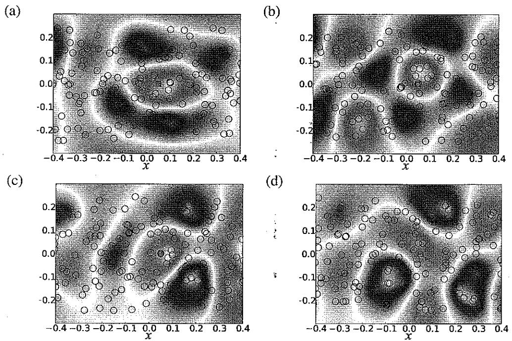
Fig. 5. Close up of scattering region of focusing for  $E_z$  polarization. (a) Magnification of central region of Fig. 4(a). (b) Central region for Fig. 4(b). (c) and (d) Central region for two other cases with same parameters but poor hot-spot behavior.
