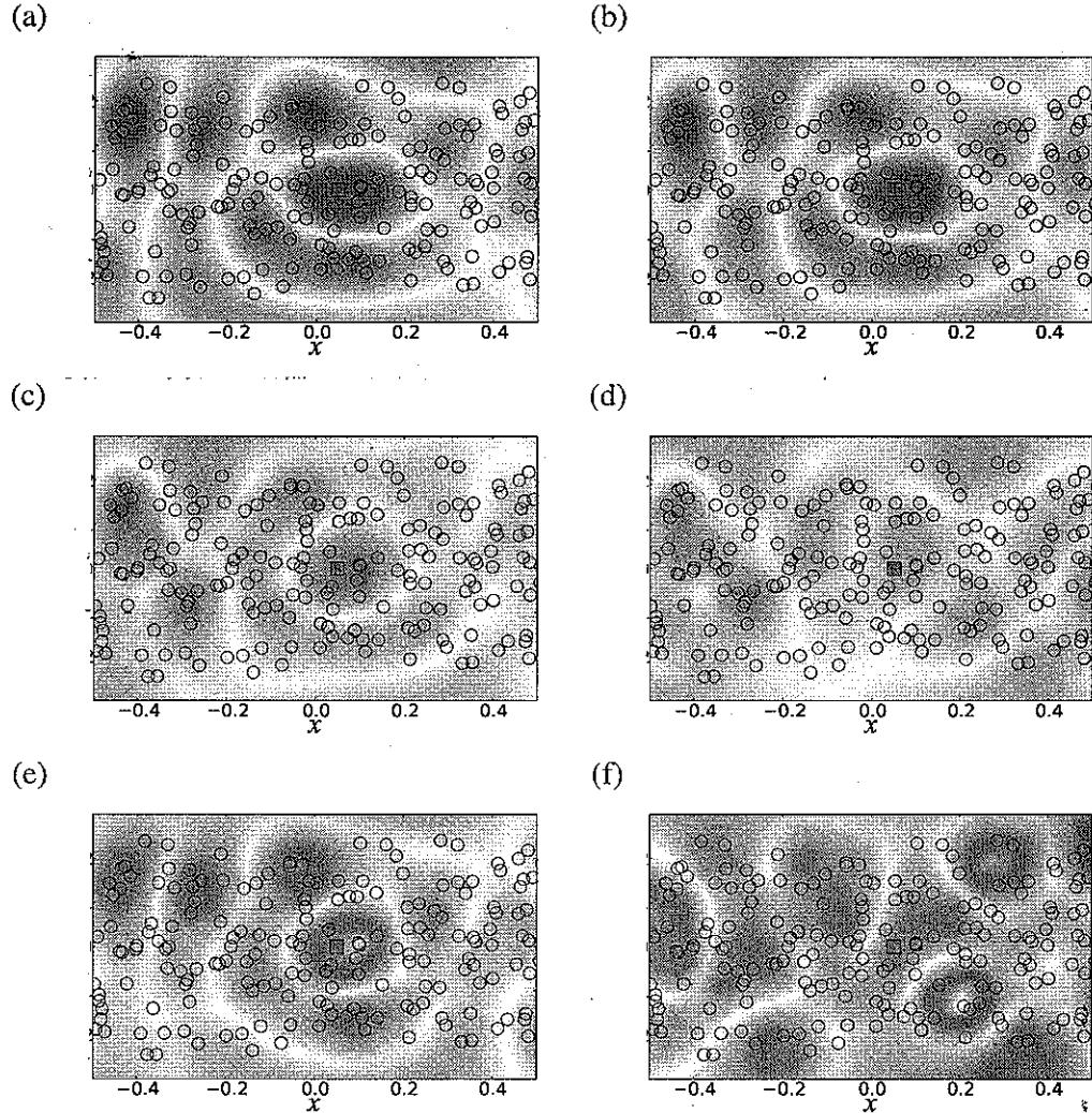
Fig. 7. Stage 2 focused field  $|E_z|$  for the scatterer configuration in Fig. 4(a) with phase noise (a)  $\eta_m = 0$ , (b)  $\eta_m = 0.75\pi$  (c)  $\eta_m = 1.5\pi$  (d)  $\eta_m = 2.0\pi$ ; and position noise (e)  $\rho_m = a/8$ , (f)  $\rho_m = a$ . The green square indicates the location of the original source.
