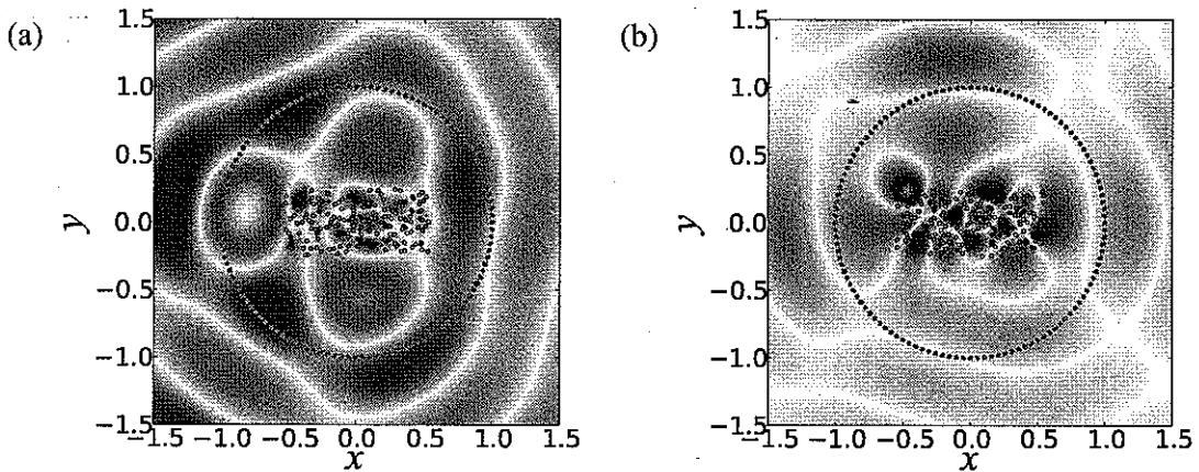
Fig. 4. Scattering domain of focusing for  $E_z$  polarization with source at  $\mathbf{r}_s = (0.05, 0)$  (green square). (a) Example with 200 scatterers of  $n_s = 6, a_s = 0.014, s = 0.0426, \tau = 0.75$ . (b) Different random arrangement with same parameters as (a).
