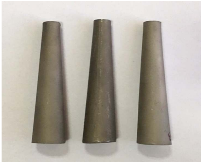
Fig. 5. Test specimens made of Inconel 713C
