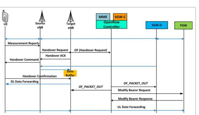
Fig. 11 Procedure for intra-GW handover with X2 support in the partial OEPC architecture
