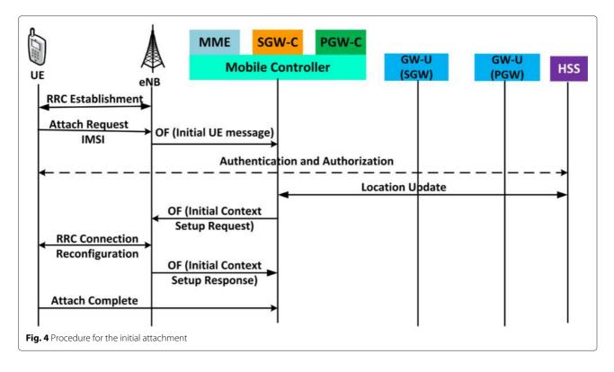
the MC needs to interact with the PCRF server through PGW-C function to get the corresponding policies before downloading the flow rules to the data plane. When the flow rules are associated with a QoS parameter, the MC will install them at the GW-Us. At the end of this procedure, the UE state is transitioned from Idle to Connected, and a data forwarding path is established from the UE to the Internet.
