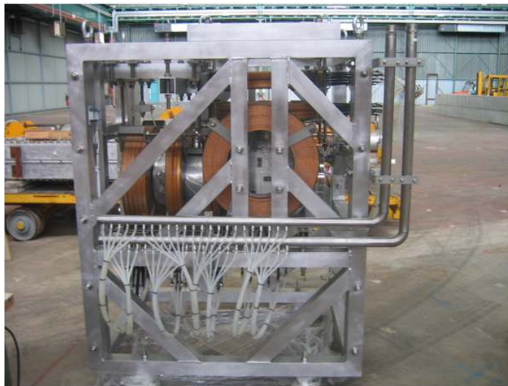
Figure 4: Photograph of the SOPHI device before its installation in front of the linac.
