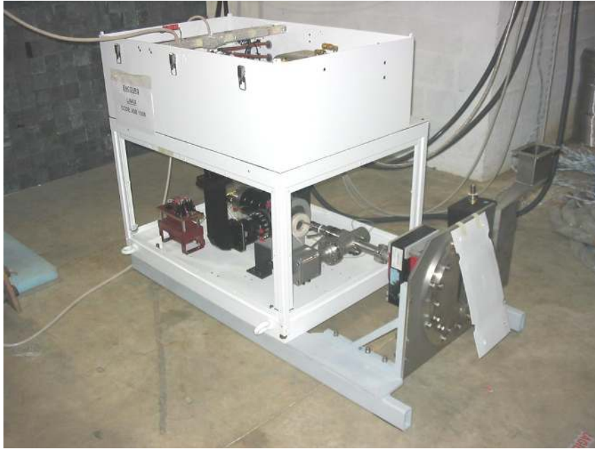
Figure 1: The 5.5 MeV demonstrator accelerator.
