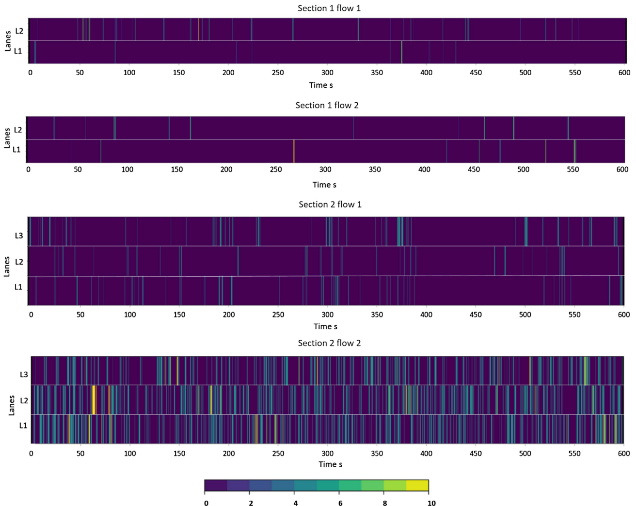
Fig. 6. Variation of string stability of lanes over time in study Sections 1 and 2.
