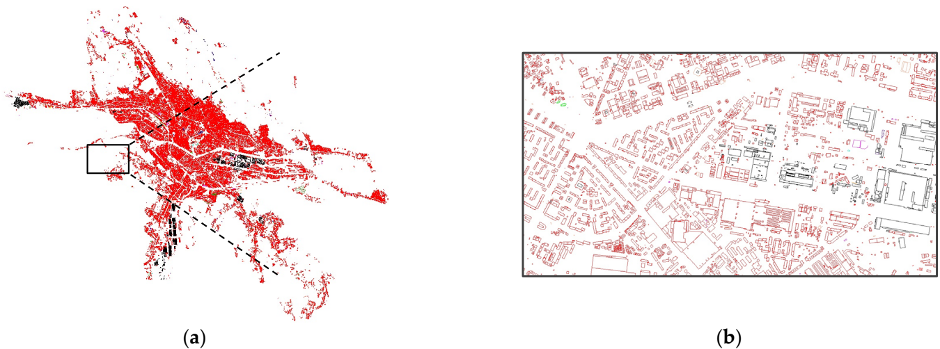
Figure 16. (a) Building sub-footprints obtained by stereo-restitution based on ADS-40 aerial images; (b) detail.
