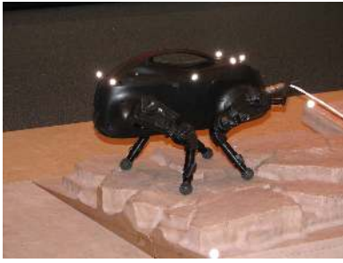
Fig. 2. The LittleDog robot (with retroreflective markers) on a terrain board.
