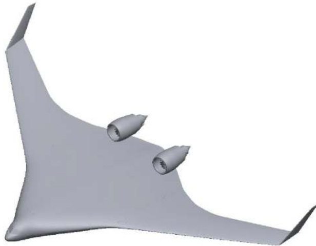
Figure 1. Schematic of a baseline, two engine Hybrid Wing Body concept based on the Boeing Blended Wing Body aircraft concept.
