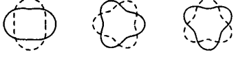
Figure 2: The variables s_1(t), s_2(t), s_3(t) correspond to 3 deformation modes. The 1 st and 2 nd modes together yield motion in the x -direction. The 1 st and 1 st modes together yield motion in the y -direction.
