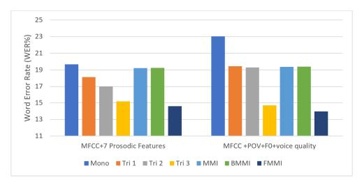
**Figure 4.** WER of integration of several prosodic features when MMI, BMMI, and fMMI discriminative technique was used.
