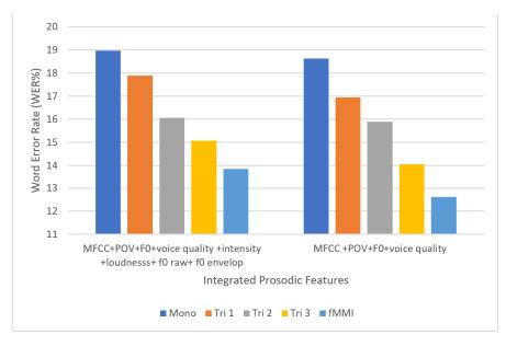
**Figure 6.** Data-augmented corpus WER of integrated prosodic features using mono, tri 1, tri 2, and tri 3 modeling and fMMI discriminative techniques.
