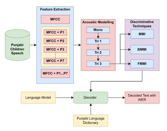
**Figure 1.** Block diagram of an implementation of discriminative techniques on the Punjabi children's speech corpus using prosodic features.
