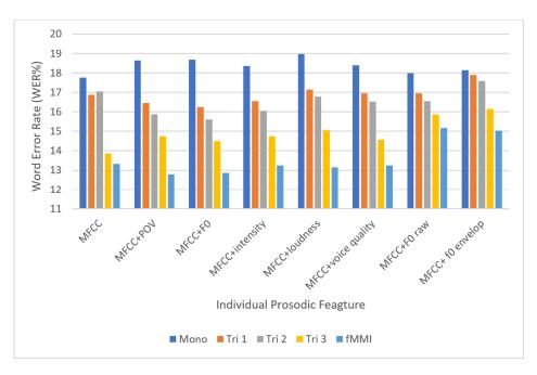
**Figure 5.** Data-augmented corpus WER of individual prosodic features using mono, tri 1, tri 2, and tri 3 modeling and fMMI discriminative techniques.
