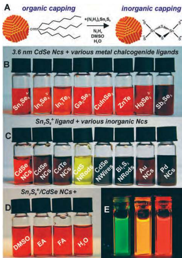
Figure 15. (A) A sketch of a generic exchange of original organic ligands by metal chalcogenide complexes: the original organic ligands (TOPO) at the surface of CdSe NC are replaced by \text{Sn}_2\text{S}_6^{4-} Zintl ions. (B) Stable colloidal solutions of 3.6 nm CdSe NCs capped with various metal chalcogenide complexes in hydrazine. (C) From left to right: stable colloidal solutions obtained by combining (\text{N}_2\text{H}_5)_4\text{Sn}_2\text{S}_6 with 3.6 and 5.8 nm CdSe NCs, 9 nm CdTe NCs, 5 \times 60 nm CdS nanorods (NRods), CdSe nanowires (NWires, \sim 25 nm wide, 2\text{--}5 \mu\text{m} long), 6 \times 25 nm \text{Bi}_2\text{S}_3 NRods, 5 nm Au NCs, and 3 nm Pd NCs. (D) From left to right: CdSe/ \text{Sn}_2\text{S}_6^{4-} NCs dispersed in dimethylsulfoxide, ethanolamine, formamide, and water. (E) Photograph of NC photoluminescence excited by a UV lamp. From left to right: 2.9 nm CdSe/ \text{Sn}_2\text{S}_6^{4-} NCs in EA (green emission, quantum yield QY \approx 2\% ), 3.6 nm CdSe/ \text{Sn}_2\text{S}_6^{4-} in DMSO (yellow emission, QY \approx 3\% ), and \text{Sn}_2\text{S}_6^{4-} -capped CdSe/CdS core-shell NRods in hydrazine (red emission, QY = 10%). Reprinted with permission from ref 273. Copyright 2009 American Association for Advancement of Science.
