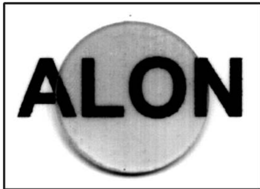
Figure 5. Fully transparent ALON sample (Cheng et al 2001a).
