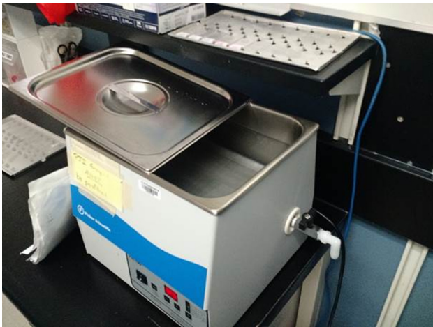
Figure 1. Ultrasonicator device used to disrupt bacterial biofilm on prosthetic and implant devices. The prosthetic device is placed in a container filled with saline and then placed in this waterbath where ultrasound waves are directed at it.
