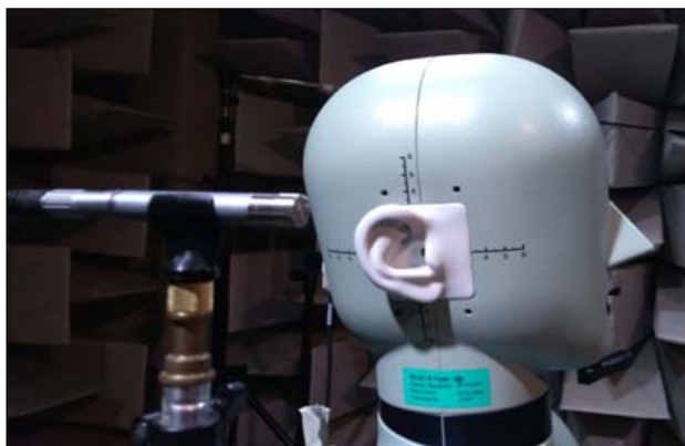
Fig. 4. The microphone n° 3 near the ear of maniquine in the chamber room
