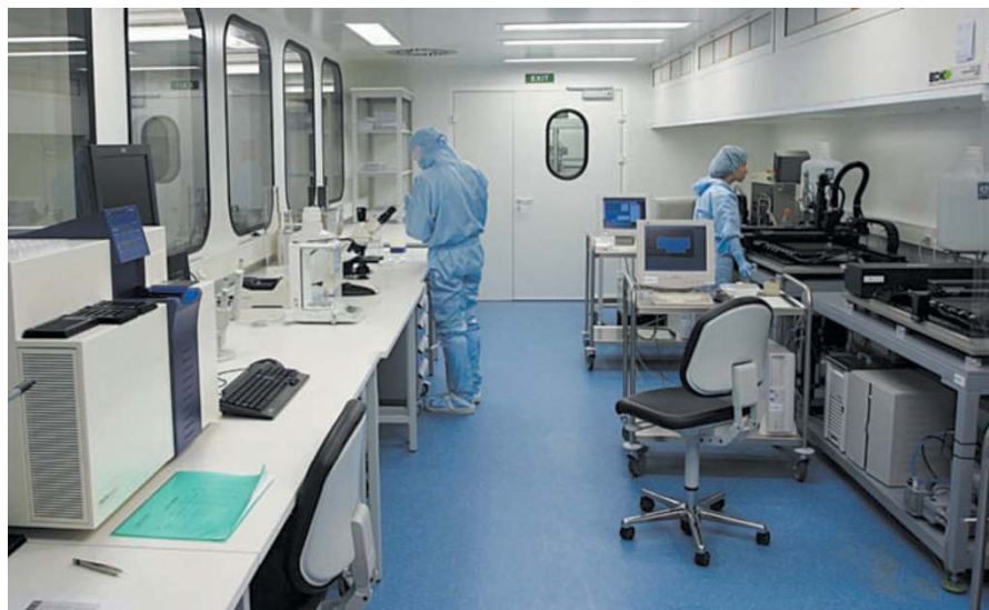
Zeptosens: microarrays must be made under rigorous clean-room conditions.
