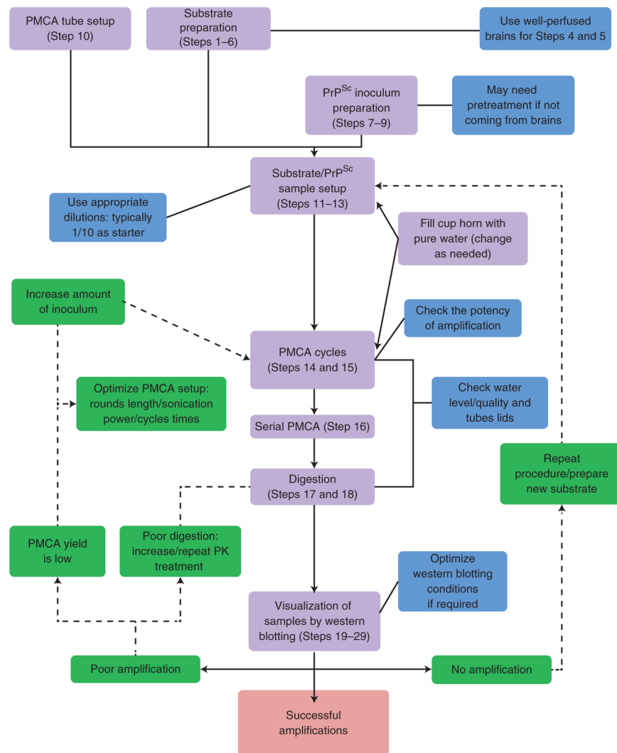
Figure 2. PMCA flowchart. A conventional PMCA assay is usually composed of four main stages: substrate preparation, inoculum preparation, PMCA procedure and visualization of the extent of prion formation. After mixing PMCA substrate and inoculum, samples are submitted to incubation/sonication cycles that will allow an exponential generation of infectious prions. After the PMCA reaction is completed, samples are digested with PK and visualized by western blotting. Modifications to this technique have been used to replicate prions from different strains/species. PMCA has been adapted for many different applications, including PrP Sc detection in body fluids and tissues and interspecies prion replication. PROCEDURE Steps are indicated in purple boxes with the step number(s) in parentheses. Critical steps are labeled in blue and Troubleshooting steps in green.
