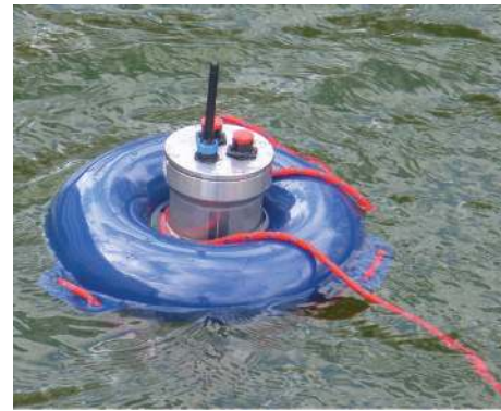
FIGURE 9: A Proteus II node deployed in the water at the test setup. The acoustic part of the node is underwater and the radio antenna is above the water surface to allow a radio connection with the gateway.
