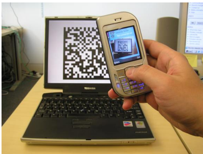
Figure 4.9: Machine visual channel: Semacode transfer from laptop to mobile phone
