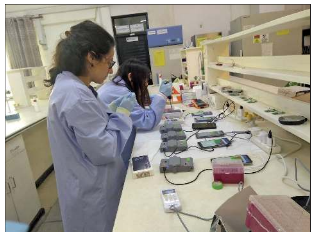
Figure 5. Validation for malaria diagnosis at the University of Ghana, Accra, Ghana. PhD students Kenny Malpartida-Cardenas and Ivana Pennisi are shown loading samples into several Lacewing devices.
