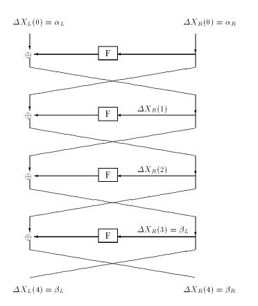
Fig. 1. The four round differential
