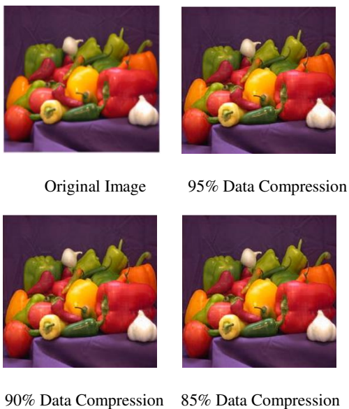
Fig 9: Shows compression of pepper image using DCT_DWT with respect to 95%, 90% and 85% of data compression.
