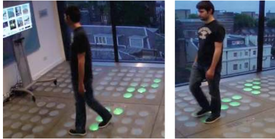
Fig. 6. Trails, visualizing the history of spatial movements of a person (Color figure online).
