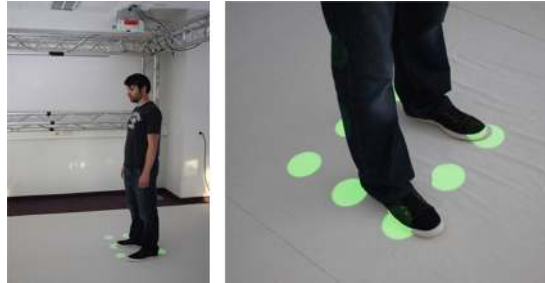
Fig. 10. Alternative floor display using a ceiling-mounted short-throw projector (Color figure online).
