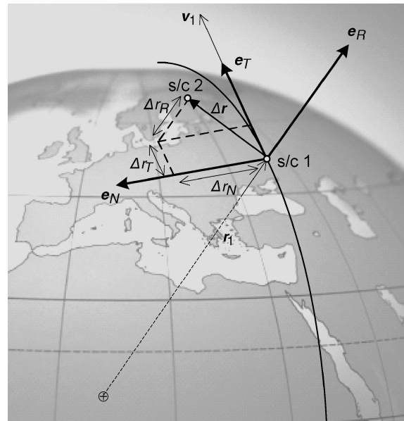
Fig. 1 Relative motion vector mapped into the orbital frame of s/c-1.
