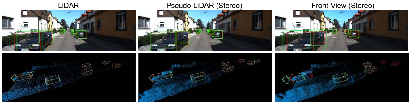
Figure 4: Qualitative comparison. We compare AVOD with LiDAR, pseudo-LiDAR, and frontal-view (stereo). Ground-truth boxes are in red, predicted boxes in green; the observer in the pseudo-LiDAR plots (bottom row) is on the very left side looking to the right. The frontal-view approach ( right ) even miscalculates the depths of nearby objects and misses far-away objects entirely. Best viewed in color.
