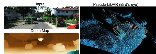
Figure 1: Pseudo-LiDAR signal from visual depth estimation. Top-left: a KITTI street scene with super-imposed bounding boxes around cars obtained with LiDAR (red) and pseudo-LiDAR (green). Bottom-left: estimated disparity map. Right: pseudo-LiDAR (blue) vs. LiDAR (yellow) — the pseudo-LiDAR points align remarkably well with the LiDAR ones. Best viewed in color (zoom in for details.)
