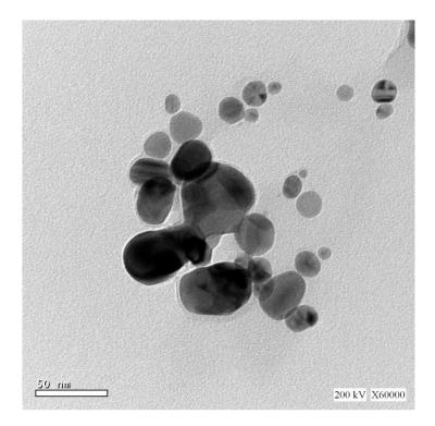
Figure 4. TEM image of AgNPs synthesized by of *P. indica* S. Azhar.
