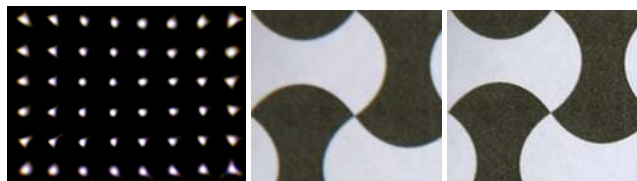
Figure 13. Chromatic Aberration. (left) The recovered spatially varying PSFs for red, green, and blue shown as a color image. The red and blue fringing is reflected in the PSF image and the PSFs are larger towards the edge of the image and spread along the direction orthogonal to the optical axis. (middle) Zoom-in on the input image. (right) After radial correction and deconvolution the aberrations are significantly reduced.
