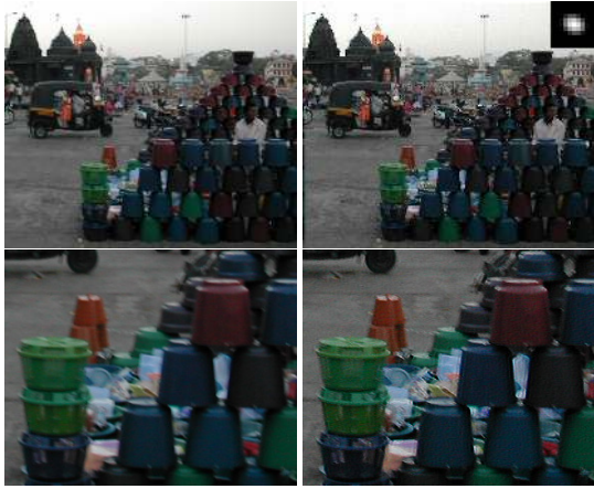
Figure 8. Motion Blur. (top row) The original blurred image (left) and the deconvolved output (right) with the recovered kernel displayed in the top right of the image (the kernel has been enlarged by 10x for display). (bottom row) Zoomed-in versions of the original and deconvolved image, respectively.
