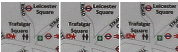
Figure 6. Kernel Size and Orientation. Image deconvolved with (left) our kernel, (middle) our kernel scaled 20% larger, and (right) our kernel rotated by 45°. The middle and right images have more ringing (most apparent at the bottom of the word “Leicester”).
