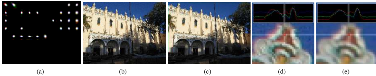
Figure 12. Blind Chromatic Aberration. (a) Recovered spatially varying PSFs for red, green, and blue shown as a color image. PSFs are only computed where there are enough edges observed. (b) The original image, (c) after radial correction and deconvolution the aberrations are significantly reduced, and (d–e) zoomed-in versions and intensity profiles for (b–c).
