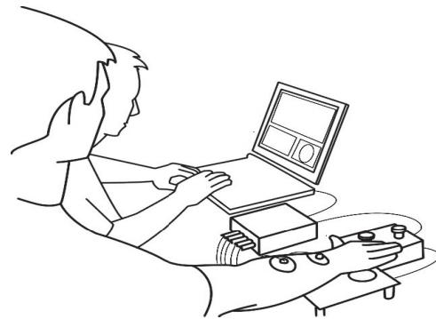
Figure 2. The subject is waiting for a tactile signal (electromagnet bolt hits against the palm).
