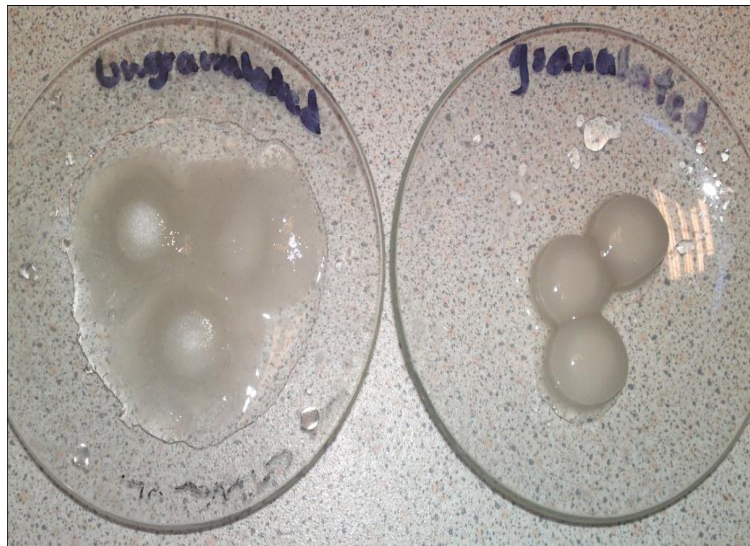
Figure 6: Comparison between 50 % Theophylline + 50 % Psyllium physical mix (ungranulated) and granulated tablets after the 12hr dissolution period. The tablets made from granulated powders maintained their integrity after the dissolution compared to the un-granulated formulations
