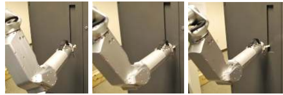
Fig. 8. Figure illustrating the two compliant motions that the robot executes to try to obtain a firm hooking grasp. Left : Starting position of the hook. Middle : Motion towards the mechanism until contact with the surface. Right : Lateral motion along the surface while pushing against it.
