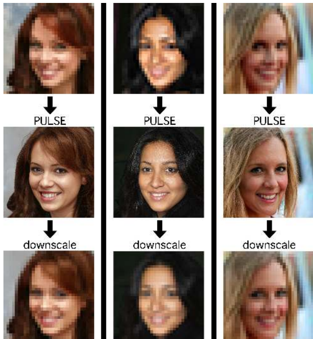
Figure 1. (x32) The input (top) gets upsampled to the SR image (middle) which downscales (bottom) to the original image.
