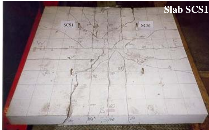
Figure 4 Crack localization in the slabs of the first phase
