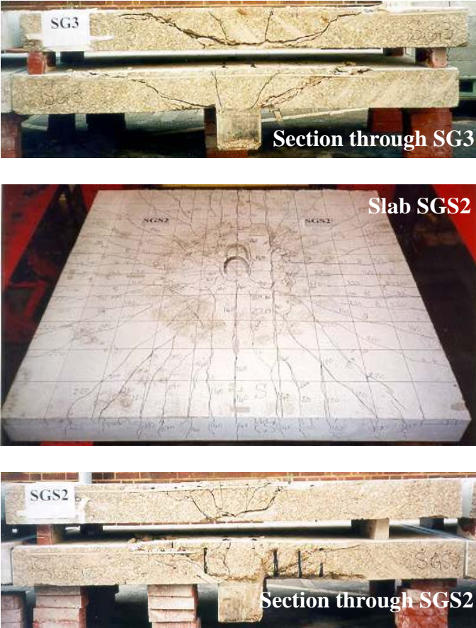
Figure 6 Punching shear failure of the slabs of the second phase
