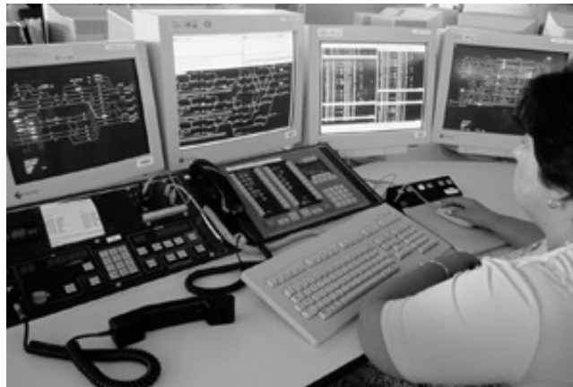
Figure 2.6 Dispatcher workplace in a centralized traffic control centre (VPT-PRL)
