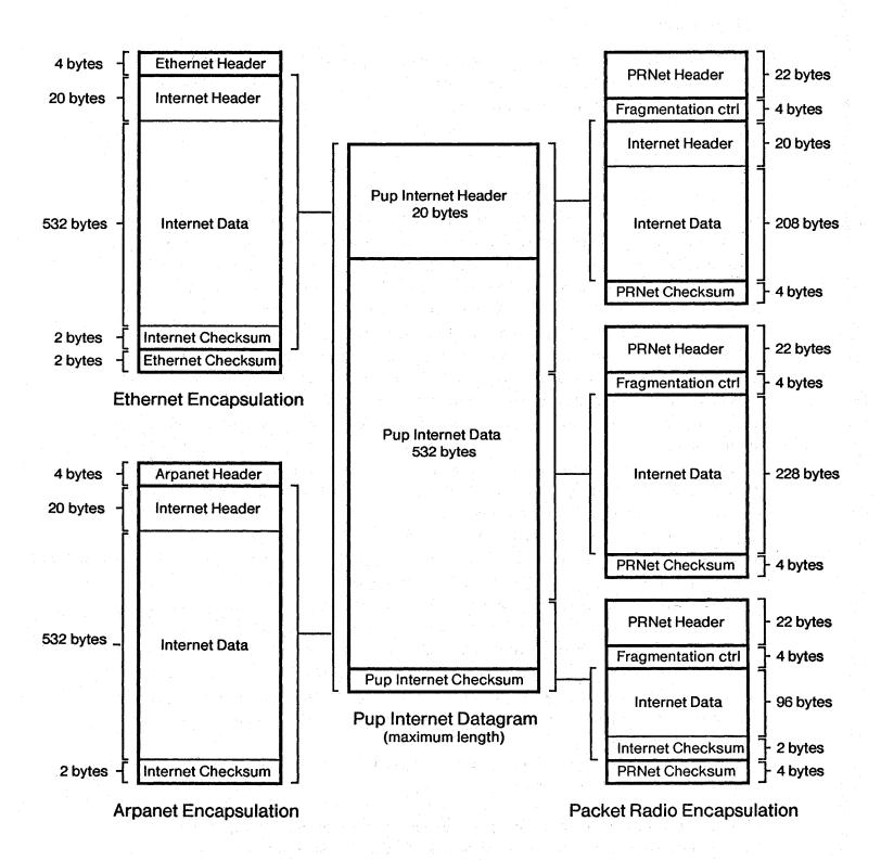
Figure 2. Pup Encapsulation in Various Networks
