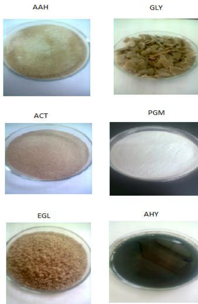
Plate 1: photographs of the pure gum arabic (PGM) and each gum modification, acid hydrolysis modified (AHY), Ethylene glycol modified (EGL), Glycerol modified (GLY), Acetolysing mixture modified (ACT), Acetic anhydride modified (AAH).
