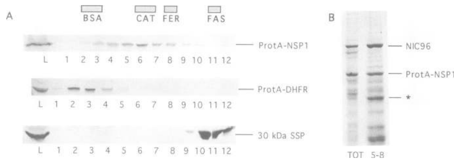
Fig. 4. Sedimentation of ProtA-NSP1 and ProtA-DHFR on sucrose gradients. (A) Cell lysates from strains ProtA-NSP1 and ProtA-DHFR, as well as a protein standard (bovine serum albumin: BSA, 66 kDa; catalase: CAT, 240 kDa; ferritin: FER, 450 kDa; yeast fatty acid synthetase: FAS, 2400 kDa) were loaded on a 7–40% sucrose density gradient and centrifuged for 17 h at 34 000 r.p.m. Each gradient was collected in 12 fractions and aliquots of the load (L) and fractions 1–12 were analysed by SDS-PAGE and Western blotting. Only the relevant area of the immunoblot containing the different fusion proteins is shown. The sedimentation of the protein standards on the gradient is indicated above the figure. In addition, the immunoblot was redecorated with an antibody recognizing a 30 kDa ribosomal protein of the small subunit (30 kDa SSP) to reveal the sedimentation of ribosomes on the sucrose gradient. (B) ProtA-NSP1 containing fractions 5–8 from the sucrose gradient were pooled and used to purify the ProtA-NSP1 fusion protein by IgG-Sepharose chromatography as described in Materials and methods. ProtA-NSP1 purified either from a whole cell lysate (TOT) or from pooled fractions 5–8 (5–8) were analysed by SDS-PAGE and Coomassie staining. The positions of NIC96, ProtA-NSP1 and a major breakdown product of ProtA-NSP1 (*) are indicated.
