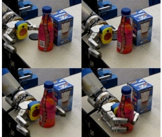
Fig. 1. An example push-grasp of an object in contact with the surrounding clutter.
