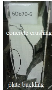
(c) Concrete crushing & plate buckling
