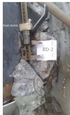
(d) Right-strip: Top branch bent down & bottom branch straightened
