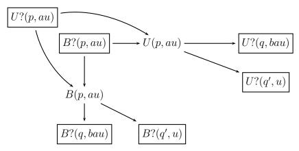
Formally, for every mode  $K \in \{B, U\}$  and for every configuration (p, u) in the pushdown game G, there is in  $G^*$  an edge from K?(p, u) to K(p, u) and to  $\overline{K}(p, u)$ , where  $\overline{K}$  denotes the "other letter". For every edge from (p, u) to (q, v) in G, there is an edge in  $G^*$  from K(p, u) to K?(q, v).
