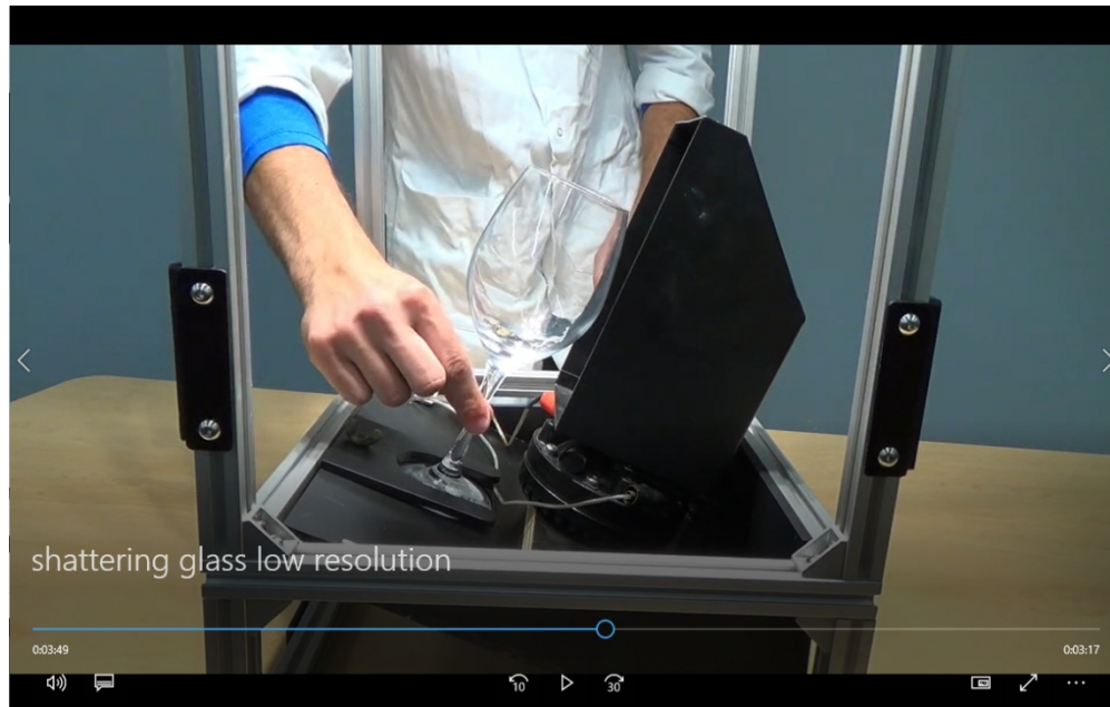
Fig. 4. The Shattering wine glass demonstration. (a) Experimental set-up; (b-d) Consequent frames of the vibrating wine glass until it breaks.
