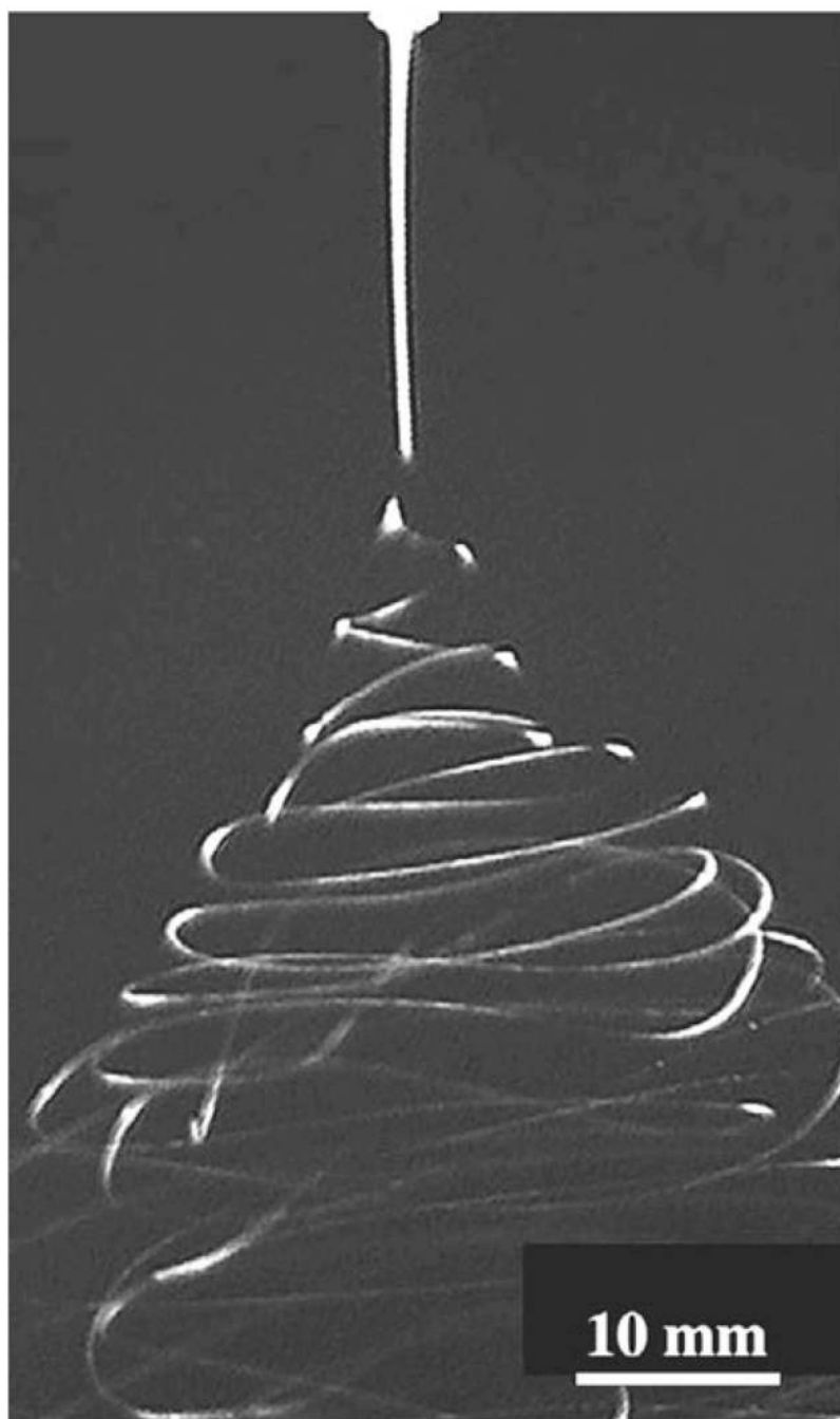
Figure 2. Photographs of typical electrospinning jets captured using a high-speed camera showing the electrically driven bending instability. Reproduced with permission from ref.[8], Copyright 2007 Elsevier.
