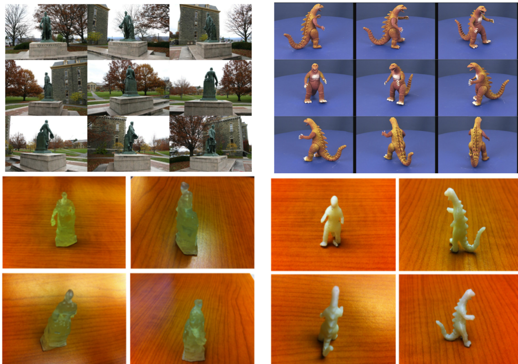
Figure 4.2: Physical 3D printout of the object of interest obtained using the proposed algorithm. The top row shows the set of multiview images of the object of interest used to obtain the 3D printout below.
