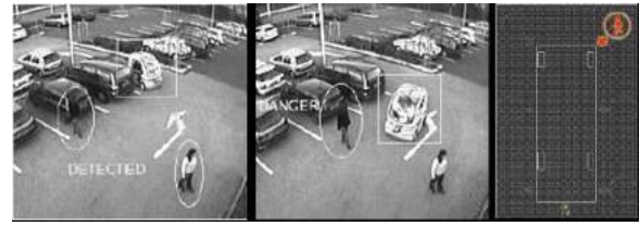
Fig. 14. (left) 2 pedestrians are crossing the road. They are detected by our system. The cycab is arriving turning right. (center) The system estimates that there is a high probability of collision between the pedestrian starting crossing the road. (right) It alerts the driver with a signal on the interface
