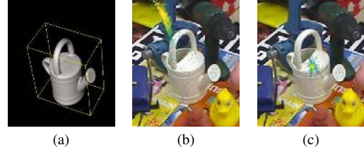
Figure 3. (a) A 3D object model and its 3D bounding box. (b) Hypotheses produced by PVNet for a bounding box corner. (c) Hypotheses produced by PVNet for a keypoint selected on the object surface. The smaller variance of the surface keypoint shows that it is easier to localize the surface keypoint than the bounding box corner in our approach.
