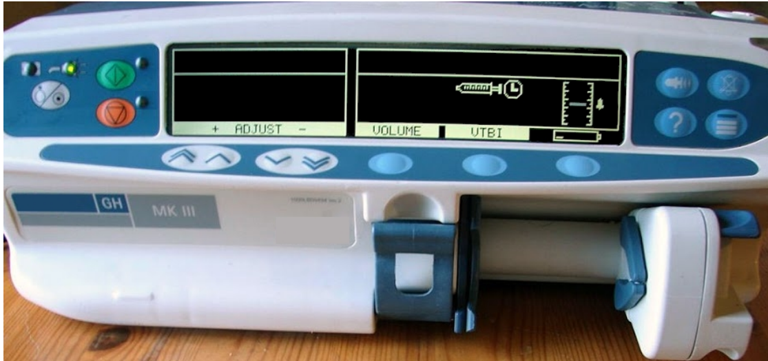
Figure 2: A picture of a commercial medical infusion pump with chevron keys.
