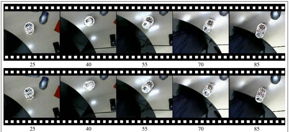
Figure 5: Film strip showing 5 frames from a video sequence of which the camera moves above the soft-drink can in a circular motion. Note that between frames 25 and 55 the view of the can moves to directly above, with the side obscured, back to a view with the side visible again. When including only the closest points as influencing the contour evolution, the pose incorrectly flips (above). In contrast the behaviour is correct when the furthest points are also considered (below).
