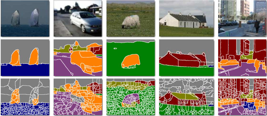
Figure 3: Several examples from the Stanford background dataset [11], where the ability of the pylon model (middle row) to choose big enough segments allowed it to obtain better semantic segmentation compared to a flat CRF defined on leaf segments (bottom row). Colors: grey=sky, olive=tree, purple=road, green=grass, blue=water, red=building, orange=foreground .
