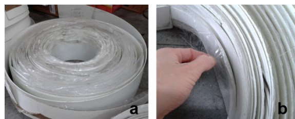
Figure 1. Typical glass fibers reinforced polyester resin laminate scraps (a) and the LDPE protective film (b)
